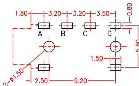
PCB Hole Layout Diagram
